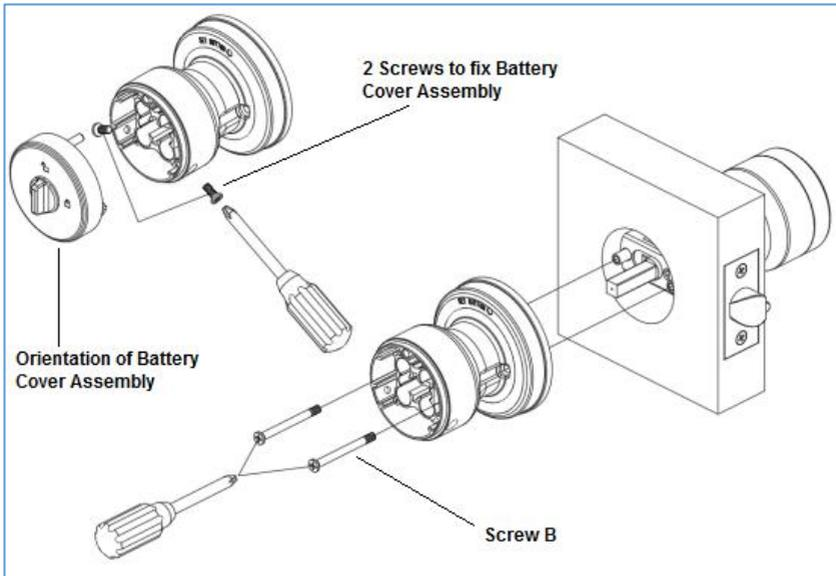
Insert Interior Knob Module by aligning the two stems with the screw holes as above image, connect the cable by inserting the connector into the socket, and drive Screw B to fix Exterior and Interior Knob Modules.
