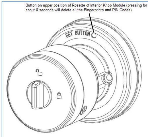
8.4. Press the Set button on the rosette of Interior Module for 8 seconds as above image, the buzzer will beep once and the Fingerprint reader will flash green. The lock will be reset to factory settings, then all the stored data will be wiped and new Fingerprint/PIN code will be required per the process of APP setting.
