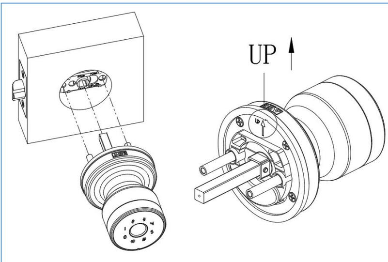
Install Exterior Knob Module (with Touch pad and Fingerprint reader) as above image from inside of your door, and make sure the Spindle and Screw Stems go through the three holes of the Latch.
