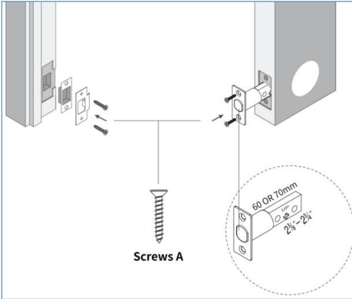
Set the backset of Latch Assembly to 2.36" or 2.76" (60mm or 70mm) to fit your door hole as above image, then insert the Latch Assembly into the door hole, and drive screw A to fix the Latch Assembly, then install Strike Box and Strike Plate with screw A into the door frame.
