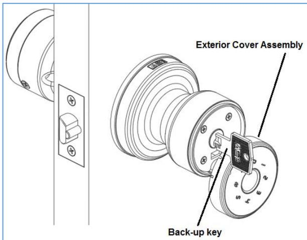
8.5. Pull the Exterior Cover Assembly of Exterior Module out and insert the back-up key to check locking/unlocking function as above image.
