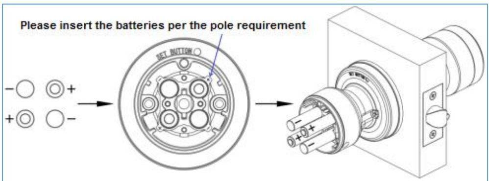
Undrive the 2 screws at side face of Interior Knob Module to dismount the Battery Cover Assembly, then insert 4 ea of AAA batteries and drive the screws to fix the Battery Cover Assembly. **Important Note:** please do not use rechargeable battery, and make sure the pole of batteries at right direction as shown by above image.
